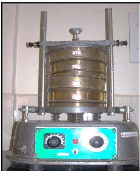
Figure 4: Mechanical sieve shaker
